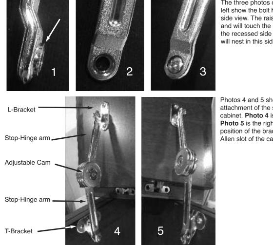
The three photos of the stop-hinge arm at left show the bolt hole. **Photo 1** shows the side view. The raised area is the pivot point and will touch the bracket. **Photo 2** shows the recessed side of the bolt hole. The bolt will nest in this side as shown in **photo 3**.
