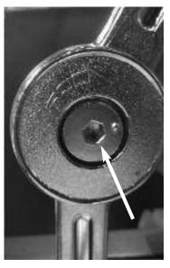
Loosen the stop-hinge by rotating the inner cam counter clockwise with the Allen wrench provided. This will allow the arms to move freely. Once the two arms are attached tighten the inner cam by rotating it clockwise. You can dampen or slow the lowering of the Flip Top by tightening the cam. Be careful not to over tighten.
